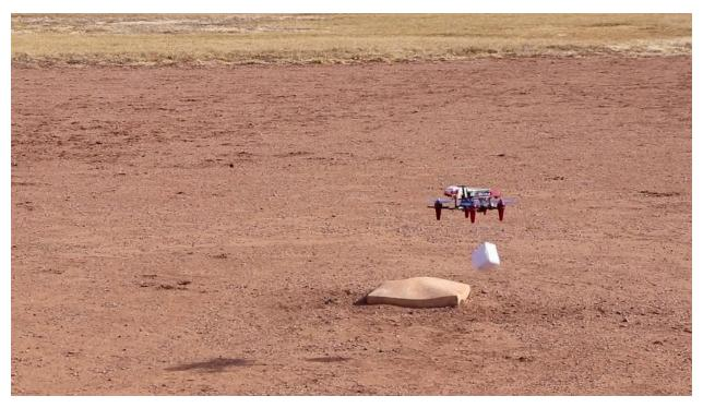
Figure 7.2. The drone releases the package at a lower altitude.
